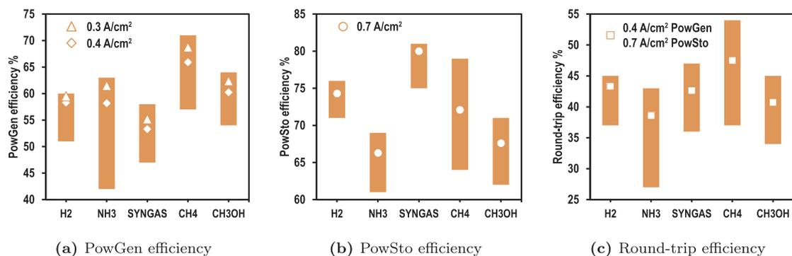
**Fig. 6.** Efficiency comparison of the process chains with the stack working at atmospheric pressure. The heat and inverter losses can lead to an efficiency drop of up to 5–10 percentage points [24]. Note that the system efficiency of the PowSto mode of the hydrogen case is reported lower than commonly mentioned by the industry, since the industrial applications usually employ waste heat from external processes for steam generation and thus need less electrical heating.
