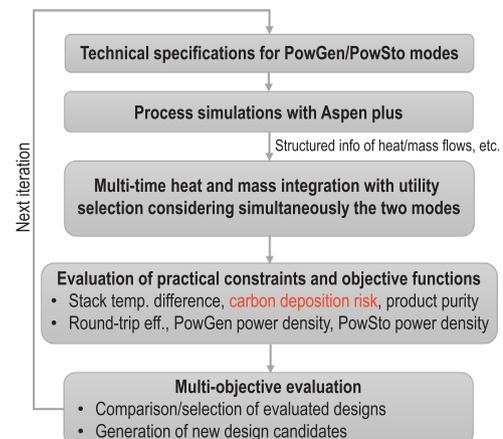
Fig. 3. Approach of optimal conceptual plant design.
